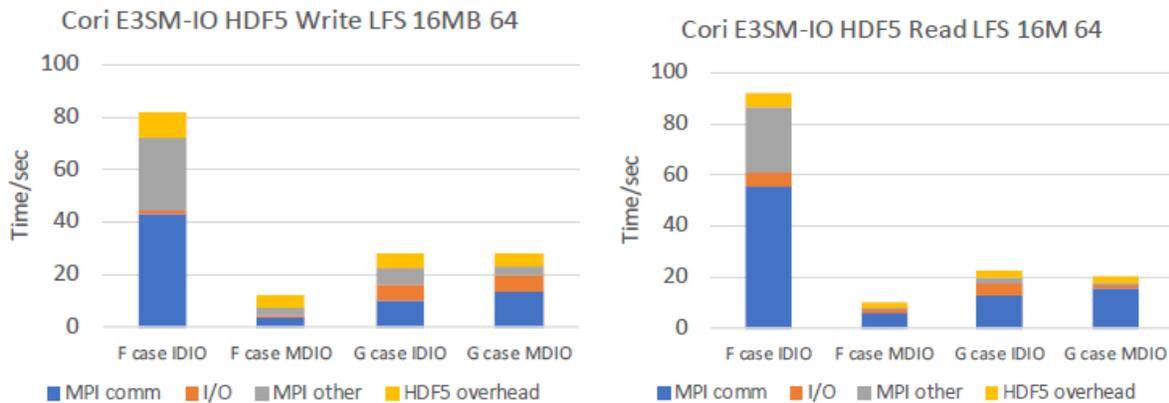
The synthetic benchmark pushes this further by increasing the number of non-contiguous blocks in the datasets, while having as many datasets as the E3SM F case and a total amount of data in between the E3SM cases. This, similarly to the E3SM F case, shows substantial performance improvement from multi-dataset I/O:
