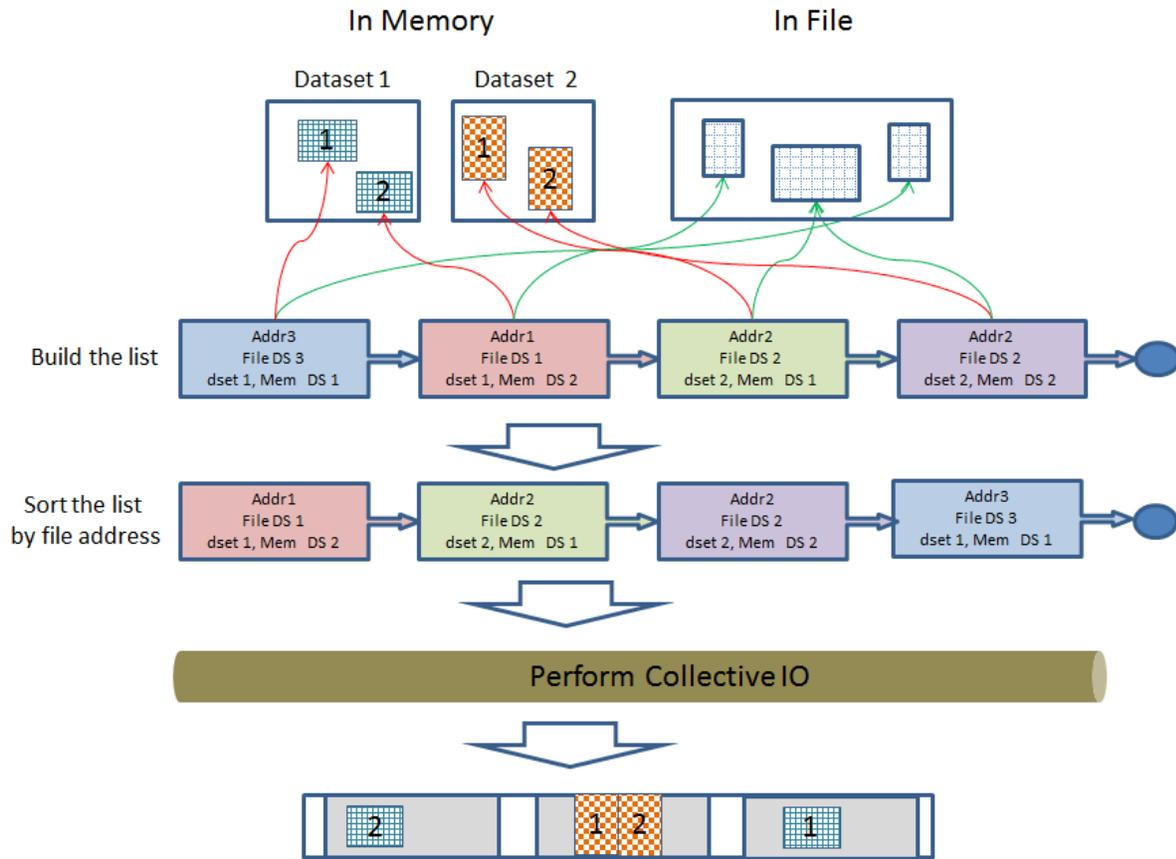
Note that sorting the list by file addresses is necessary because MPI requires the file type to consist of derived datatypes whose displacements are monotonically non-decreasing.
