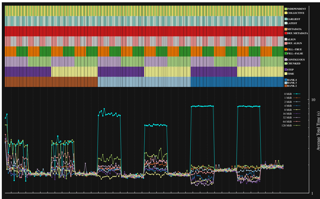
Figure 16 Total time (read and write) for all elements in the HDFspace set for ANL 144 ranks, with no delay for a compute phase and various sizes of automatic chunking. The performance degrades when turning off or making the chunk size too large.
