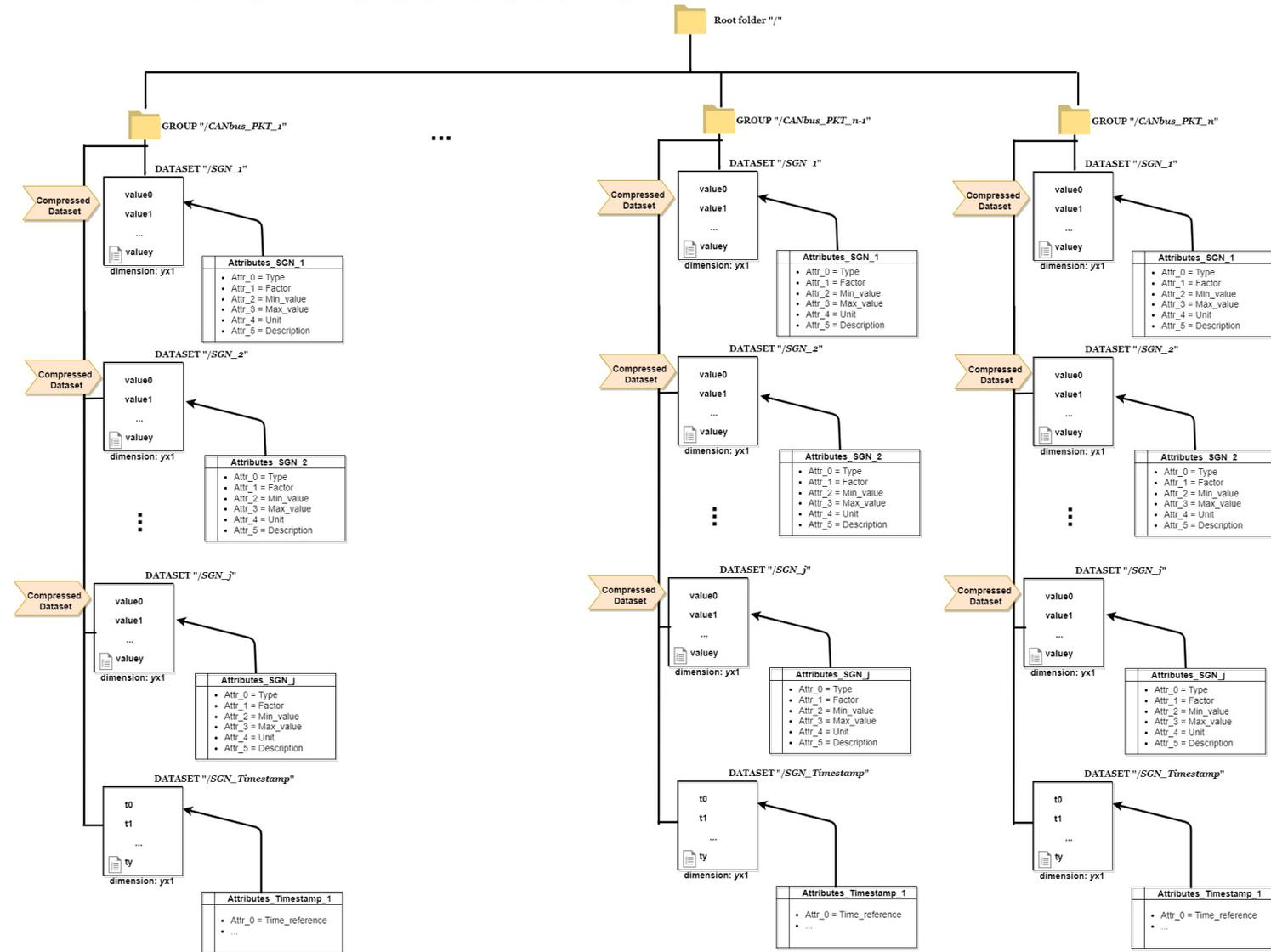
Each CAN packet has a variable number of information (so called signals) inside. Each packet travels on the bus with its own sample rate and the data recorder must follow them and store the correct acquisition time for a right post-analysis.
