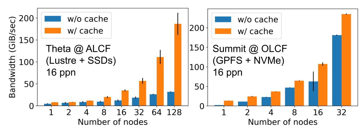
Parallel read performance. The bandwidth is averaged over four iterations. At each step, the application reads a random batch (32) of samples (224x224x3) with shuffling. The application reads through the entire dataset in one iteration.
