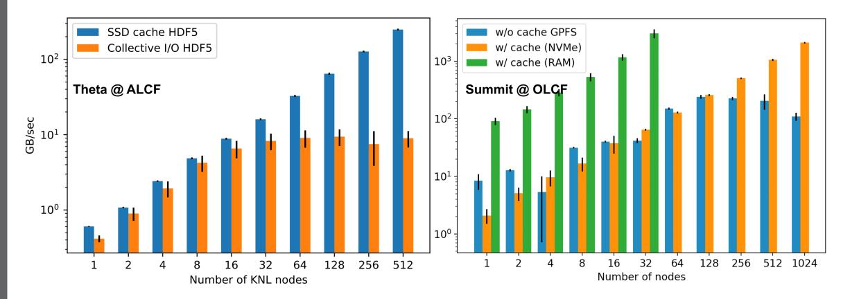
Parallel write performance: each process writes 16MB of data to a shared HDF5 file. The type of node-local storage is either SSD/NVMe or RAM. With caching, the write bandwidth scale linearly with a larger aggregate bandwidth surpassing the Lustre / GPFS write bandwidth.
