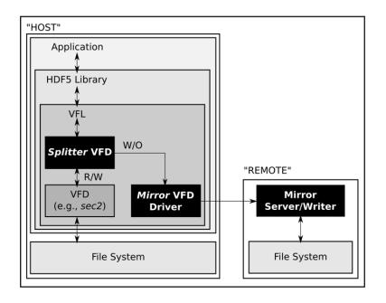
Duplicates all writes to the local HDF5 file on the remote system. Mirror server must run on the remote server.
